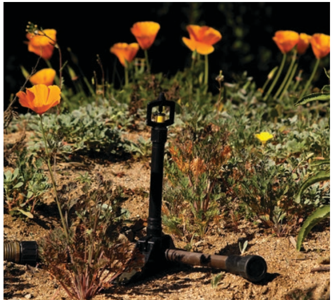
Hose-end mini sprinkler with 9 - foot radius supplies approximately 1/4” precipitation per hour, ideal for cycle/soak or pulse irrigation deep soak.
