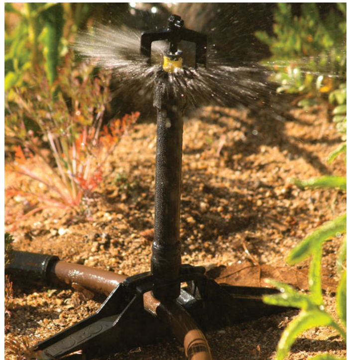
A mini-sprinkler applies water very slowly, approximately 1/4" per hour. The droplets are very small and the water effectively soaks into the ground. Use care to not wet the leaves for prolonged periods during hot weather. Adjust the flow for wind. If you see mist rising from the sprinkler head, turn the water down.
