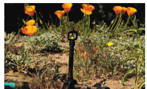
A mini-sprinkler like this one attaches to a hose and applies water very slowly, approximately 1/4" per hour. The droplets are very small and the water effectively soaks into the ground.
